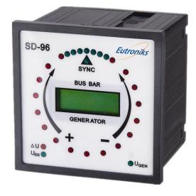
Show the phase difference and frequency difference between the two grid system and the generator. The frequency and voltage of the two grid system are close to the same, and the LED of the meter will show a slow rotation, SYNC indicates the area LED lights, closing the grid.
